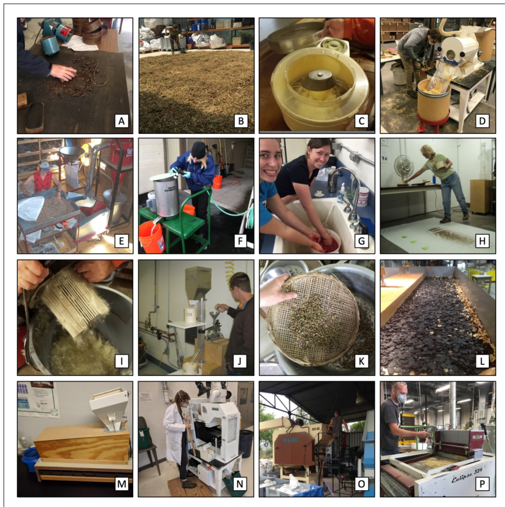
Figure 1. Techniques and equipment frequently used in seed processing. I. Seed extraction: A. Gentle beating, rolling, or manual separation from attached fruits or florets (S. Frischie/USDA Beltsville Plant Materials Center, U.S.); B. Exposure to warm or dry temperature to open dehiscent fruits (C. Galvez/Semillas Silvestres, S.L., Spain); C. Mortar/cement mixers, rock tumblers, kitchen blenders, or food processors with plastic blades (M. Skinner/Skinner Native Seeds, Canada); D. Brush machine or debearder (USDA Forest Service Bend Seed Extractory, U.S.); E. Hammer mill (B. Kleiman/Nachusa Grasslands, U.S.); F. and G. Macerators or grinders (USDA Forest Service Bend Seed Extractory, U.S.); II. Separation of seed from undesirable material: H. Fan (USDA Forest Service Bend Seed Extractory, U.S.) I. Vacuum (M. Skinner/Skinner Native Seeds, Canada); J. Continuous seed blower (USDA Forest Service Bend Seed Extractory, U.S.); K. Sieves and screens (S. Frischie); L. Gravity table (USDA Forest Service Bend Seed Extractory, U.S.); M. Velvet roller mill (Laura Fischer Walter, Tallgrass Prairie Center, University of Northern Iowa, U.S.); N. Air screen cleaner or fanning mill (Laura Fischer Walter, Tallgrass Prairie Center, University of Northern Iowa, U.S.) O. Air screen cleaner or fanning mill (S. Frischie/Semillas Silvestres, S.L., Spain); P. Air screen cleaner or fanning mill (USDA Forest Service Bend Seed Extractory, U.S.). Other types of equipment, not pictured: thresher, acid digestion, flash flaming, manual separation, indent cylinder, spiral separator, color separator, aspirator, blower.
